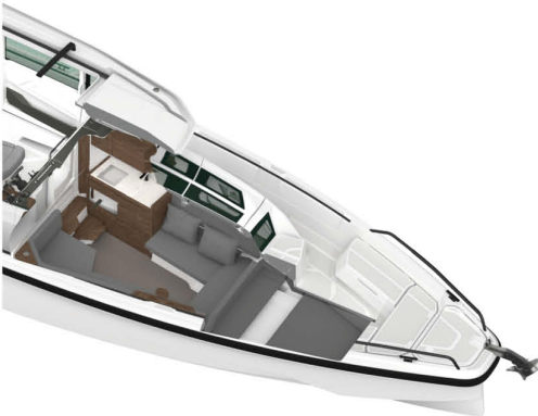
Standard configuration with pentry module and hidden toilet.
