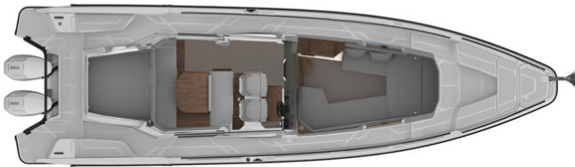
Standard aft sofa with bench seat, fixed table leg, and two rotating helm seats.
